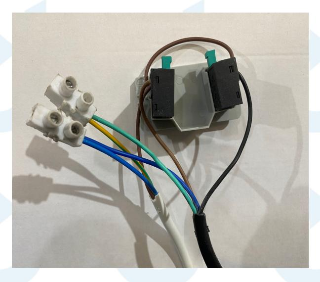
The BLACK and BROWN wires coming from the motor are directional wires, so may need to be swapped over if the operational direction is incorrect. (i.e up button taking the door down & vice versa)
