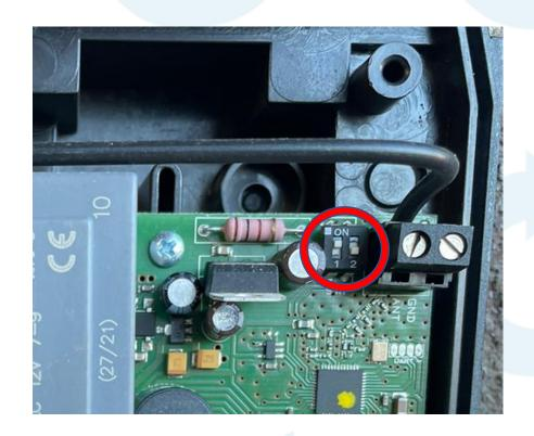
To alter the dip switches this must be done within 30 seconds of powering on the control panel
